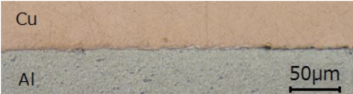
Fig.7 Optical micrograph of weld interface at one weld zone.
