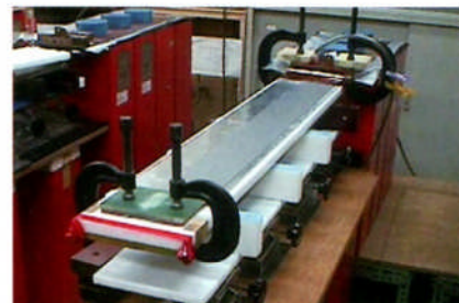
(b) Sheets for welding put on insulated above coil.
