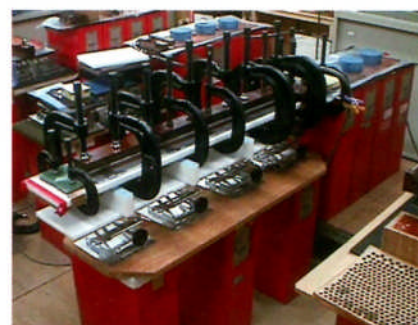
(c) Fixation of coil and sheets with clamping vises.
