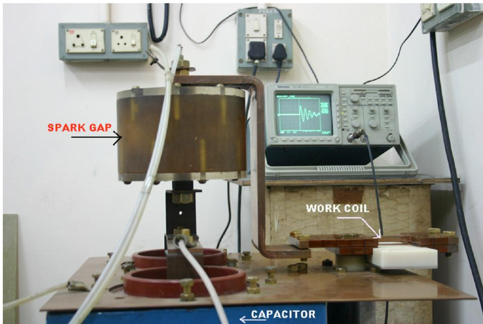
Fig. 2. Experimental setup for electromagnetic impact welding.
